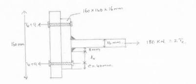
3. Calculate the size of weld for the bracket shown in figure below.
